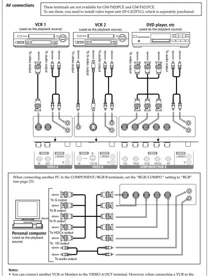
Vou can connect another VCR or Monitor to the VIDEO A OUT terminal. However, when connecting a VCR to VIDEO A terminals, do not connect both IN and OUT terminals to the same VCR.
