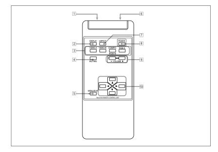
1 Remote control cable jack (page 11) Connect the remote control cable (not supplied) when using this remote control as a wired remote control.
